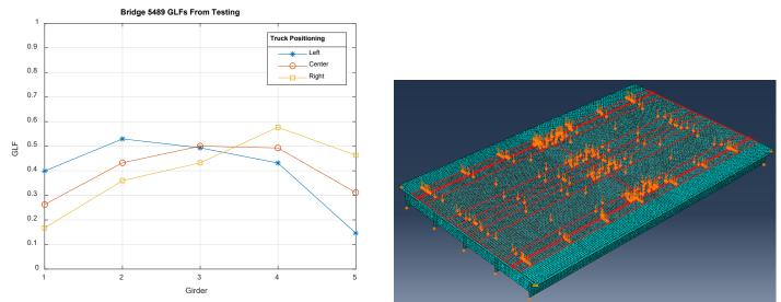
(Left: Load distribution analysis of a skewed T-beam bridge showing non-uniform distribution as loads are shifted transversely; Right: Proxy Finite Element model of an un-skewed T-beam bridge showing finite element mesh and live-loading)
