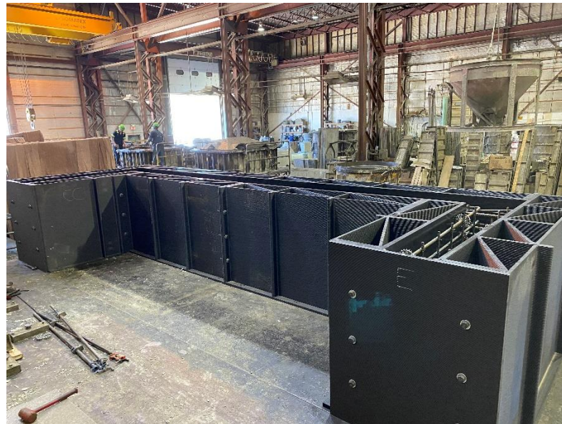
Figure 1 – Large-scale railroad bridge ballast retainer formwork at American Concrete plant in Veazie, Maine.
