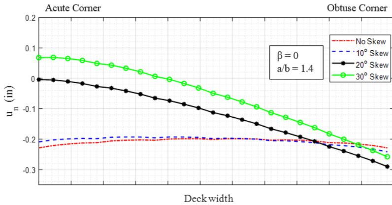
**Fig. 2** Normal horizontal displacement behind the abutment wall near the deck level for a single span sample IAB for a range of skew angles under thermal expansion for  $a/b=1.4$  and  $\beta=0$  (the results of the parametric study)
