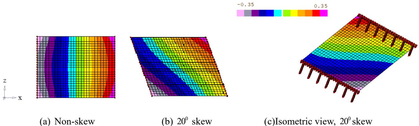
**Fig. 3** Displacement contours for a sample single span IAB under thermal expansion for  $a/b=1.4$  and  $\beta=0$
