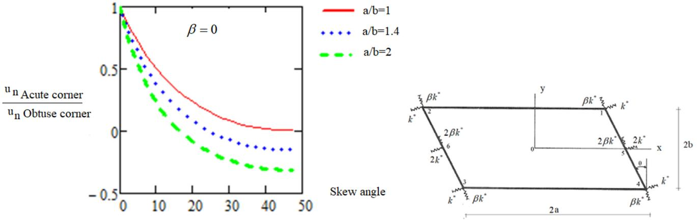
**Fig. 1** Variation of the ratio of normal displacements at the corners of the plate for a range of skew angles under thermal expansion for ranges of  $a/b=1, 1.4, 2$  and  $\beta=0$  (the results of the analytical study)
