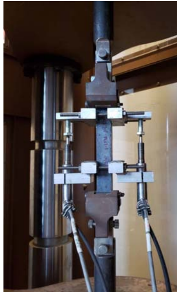
Fig:- Direct Tension Test Setup
