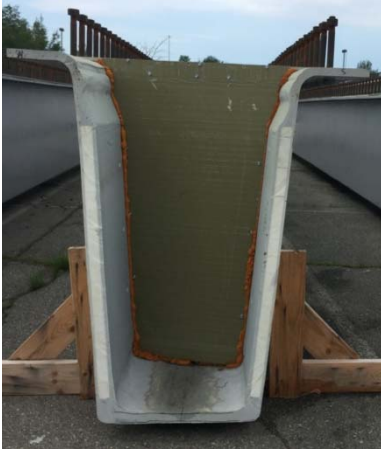
Figure 9. Composite bridge girder at AIT Bridges (Brewer, ME)
