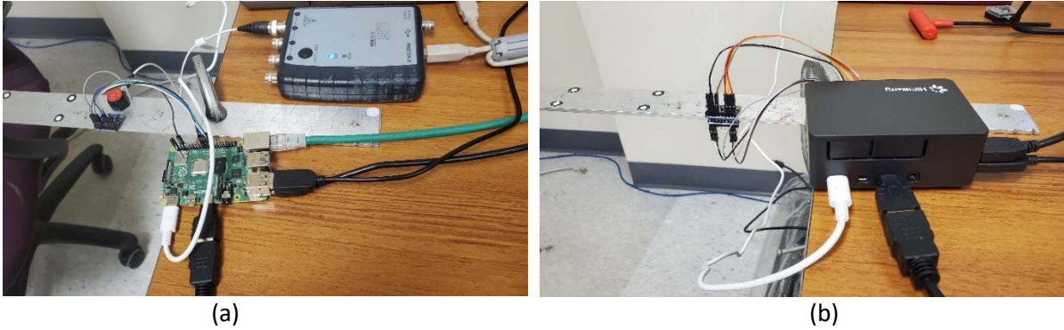
Figure 2. Setup of the lab-scale test of ground motion compensation (a) comparing ADXL345 with PCB accelerometer and (b) using two ADXL345 back-to-back
