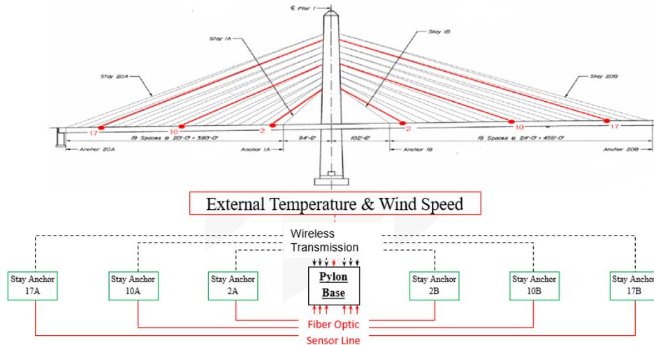
Figure 1: Data acquisition layout for carbon fiber composite strands in the Penobscot-Narrows Bridge
