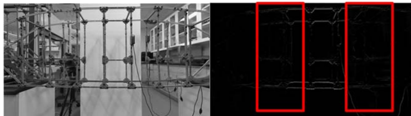
Figure 2. (a) Frame of the bridge, (b) frame of the bridge after background removal.
