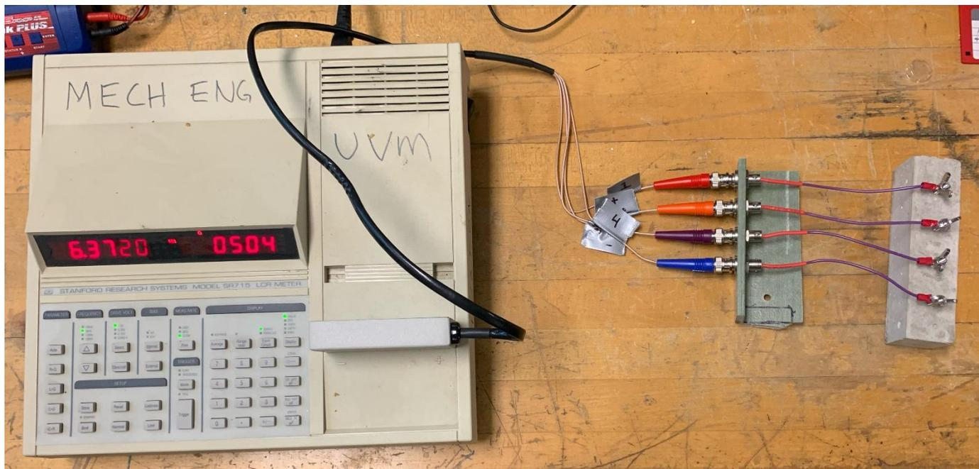
**Figure 2.** Impedance analyzer with 4-point Kelvin probe configured to take electrical surface resistivity measurements of concrete samples with a Wenner probe configuration.
