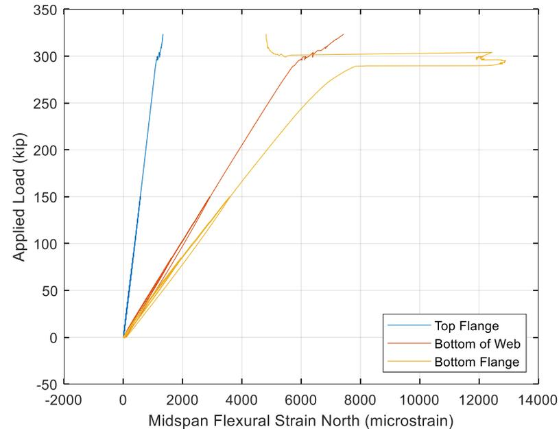
Figure 2: CT girder ultimate loading midspan strain
