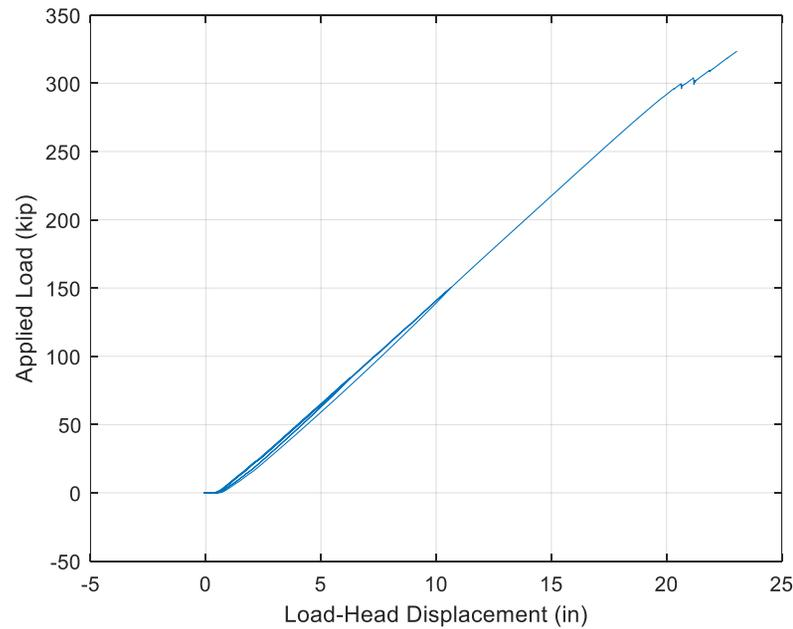
Figure 1: CT Ultimate Load-Displacement Behavior
