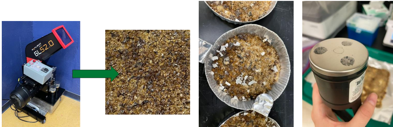
Glass crusher and lab manufactured processed glass aggregate (LM-PGA), LM-PGA samples post-furnace process, metal collected from LM-PGA
