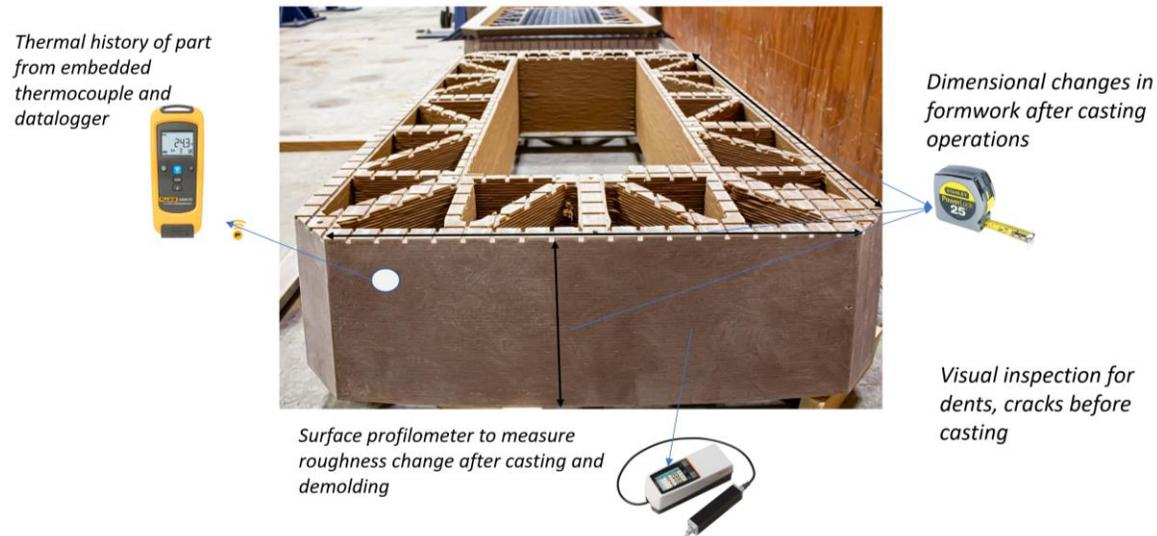
Figure 1 – Methods to monitor the formwork quality during casting and after each casting cycles.
