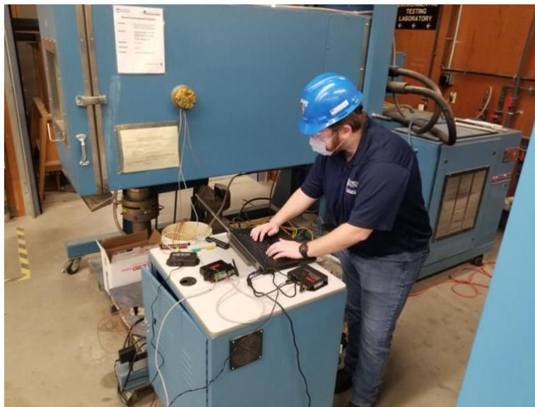
Figure 1 Graduate student Braedon Kohler working on temperature verification of the data acquisition system for sensors in an environmental chamber in the lab
