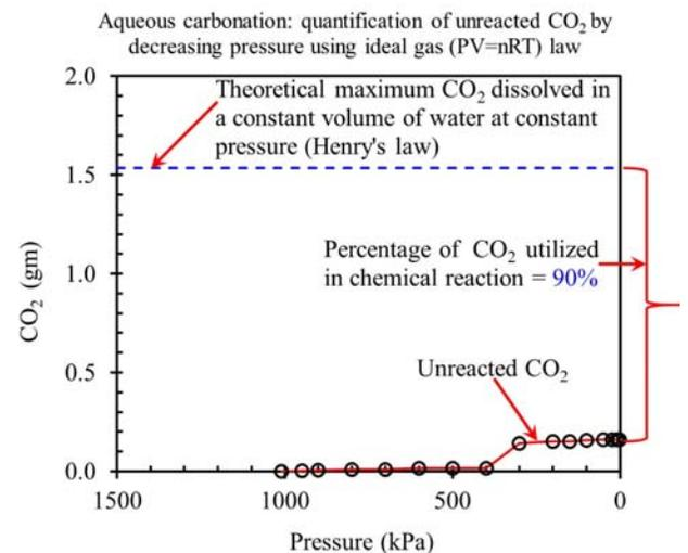
Figure 2. Carbon dioxide (CO<sub>2</sub>) gas utilization when 100 cm<sup>3</sup> of carbonated water passed through the specimen under 1 MPa pressure
