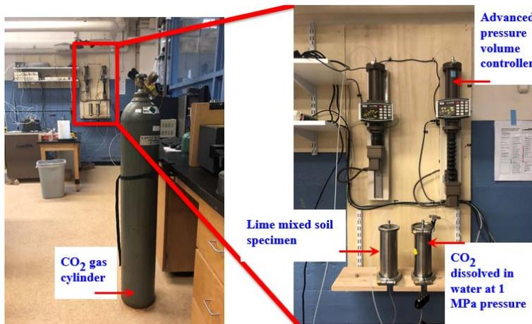
Figure 1. Laboratory test setup for aqueous based soil carbonation
