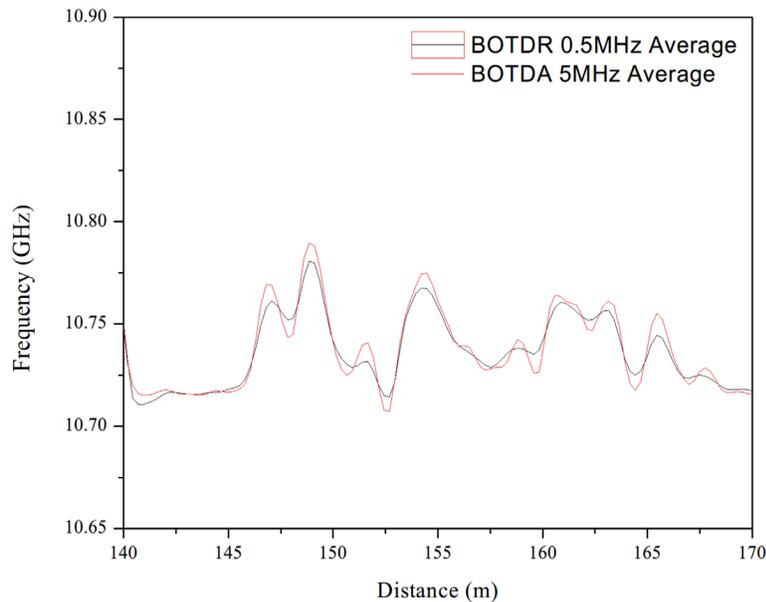
Figure 2 Comparison between BOTDA and BOTDR results.
