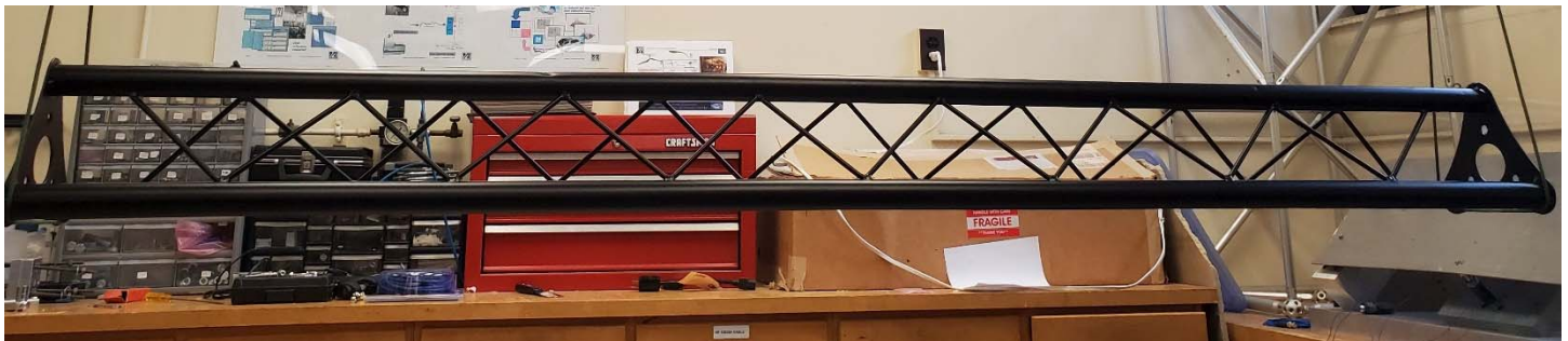
Figure 4. Metallic truss structure for future testing.
