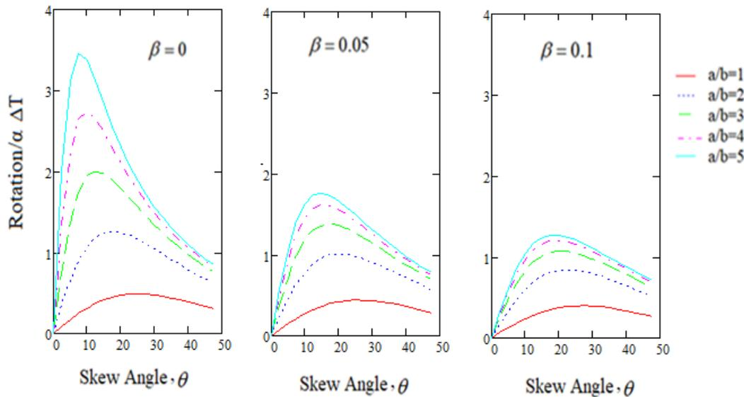
Horizontal variation of in-plane rotation of rigid plate for a range of skew angles and a range of relative stiffness of wing wall ( $\beta=0, .05, .01$ )
