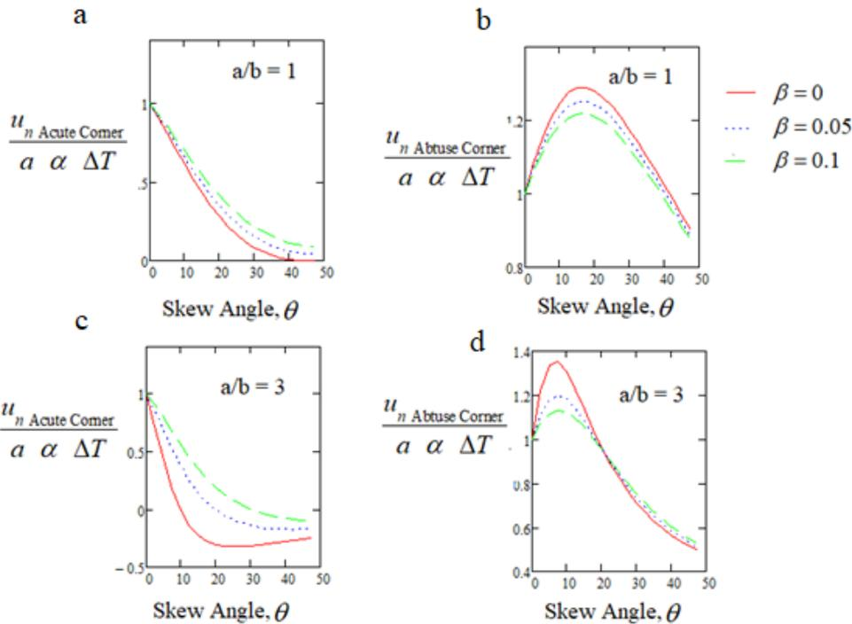
Horizontal variation of normal displacements of rigid plate for range of skew angle ( $\alpha$ ) and range of relative stiffnesses of wing wall ( $\beta=0, .05, .01$ ). (a) Acute corner, Length/width=1. (b) Obtuse corner, Length/width=1. (c) Acute corner, Length/width=3. (d) Obtuse corner, Length/width=3
