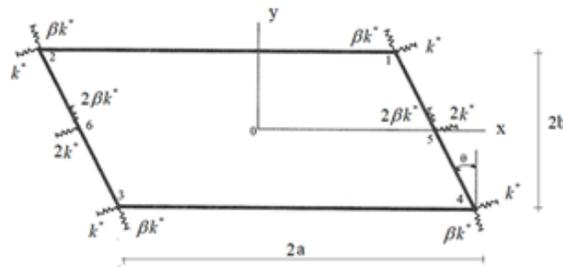
Geometry of a skew plate and location of springs
