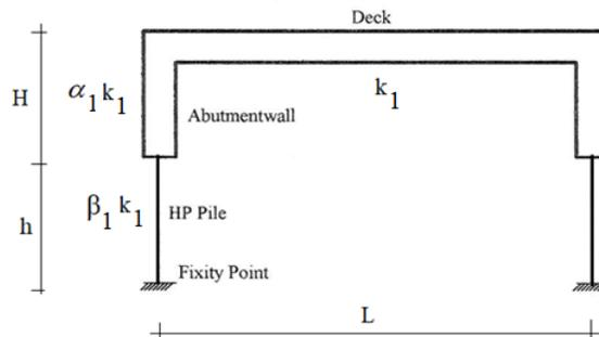
**Single story rigid frame representing a single span non-skew IAB**
