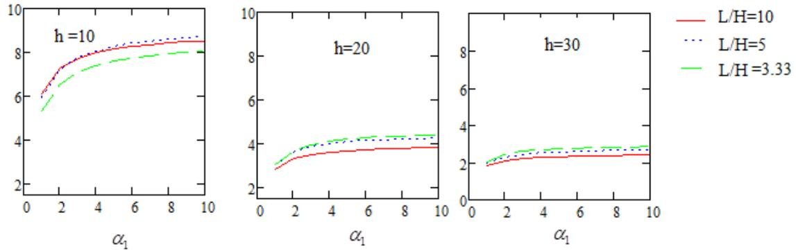
Moments at the junction of the horizontal and vertical members of the rigid frame under thermal loading for a range of relative stiffness  $\alpha_1$
