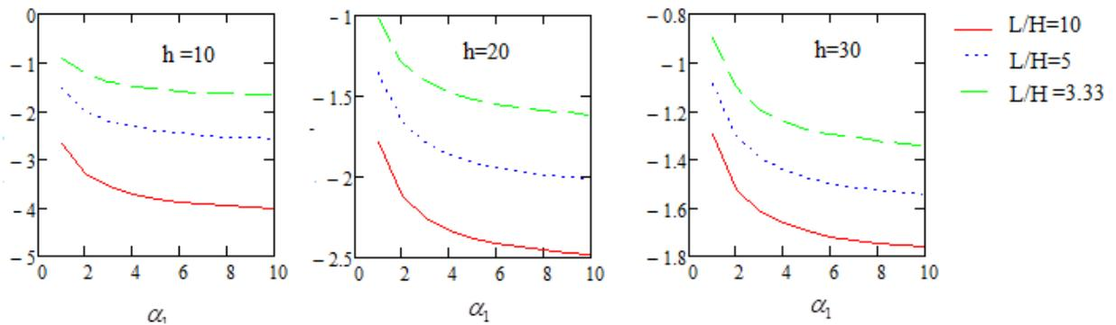
Moments at the junction of the two vertical members of the rigid frame under thermal loading for a range of relative stiffness  $\alpha_1$
