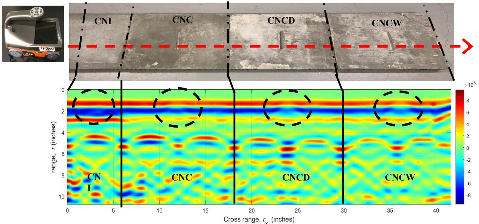
In the last report, we provided the information on series of image processing techniques to detect the crack in artificially cracked specimens CNI, CNC, CNCD and CNCW using the 1.6 GHz portable ground penetrating radar (GPR). In this report, we formulate the mathematical model to calculate the depth of an artificial crack on concrete panels. Fig. 1 shows the 1.6 GHz GPR and the B-scan GPR images of intact and artificially-cracked
