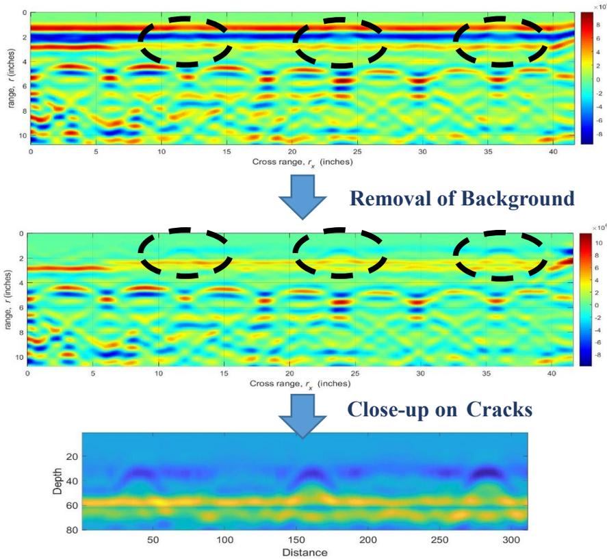
**Fig 2:** Processed GPR B-scan images
