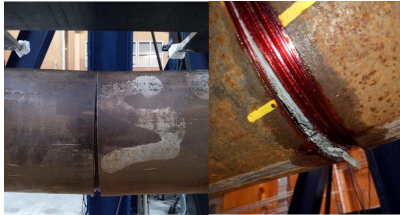
Figure 2 Detail of failed connections
