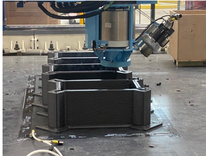
Figure 1 – 3D printing of CF-ABS formwork
