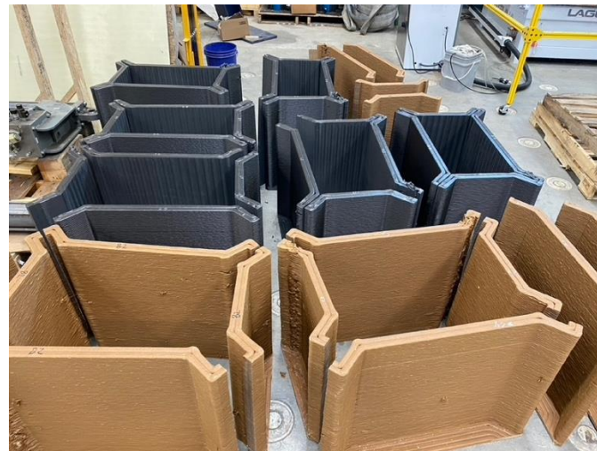
Figure 2 – CF-ABS and WF-aPLA formwork parts
