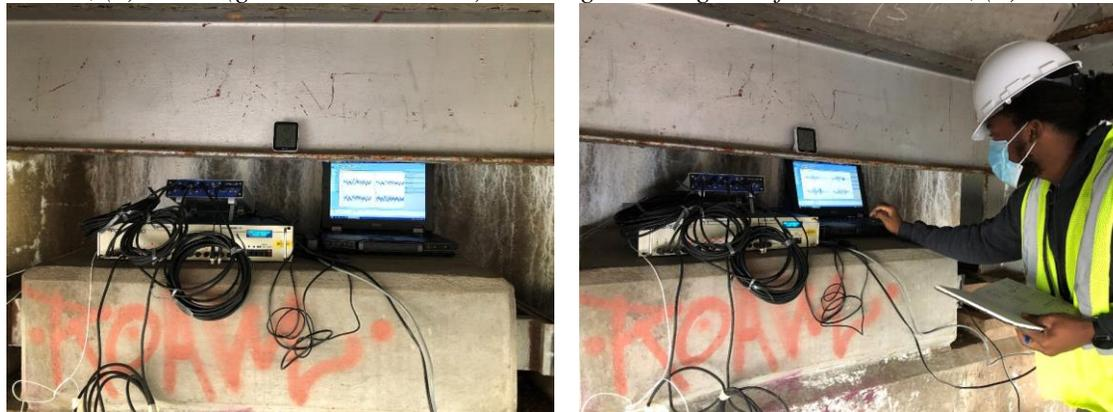
*Figure 4. Wired Acceleration Data Acquisition System with a reference temperature/humidity sensor (a) system, (b) Pierre (graduate researcher) checking the data.*
