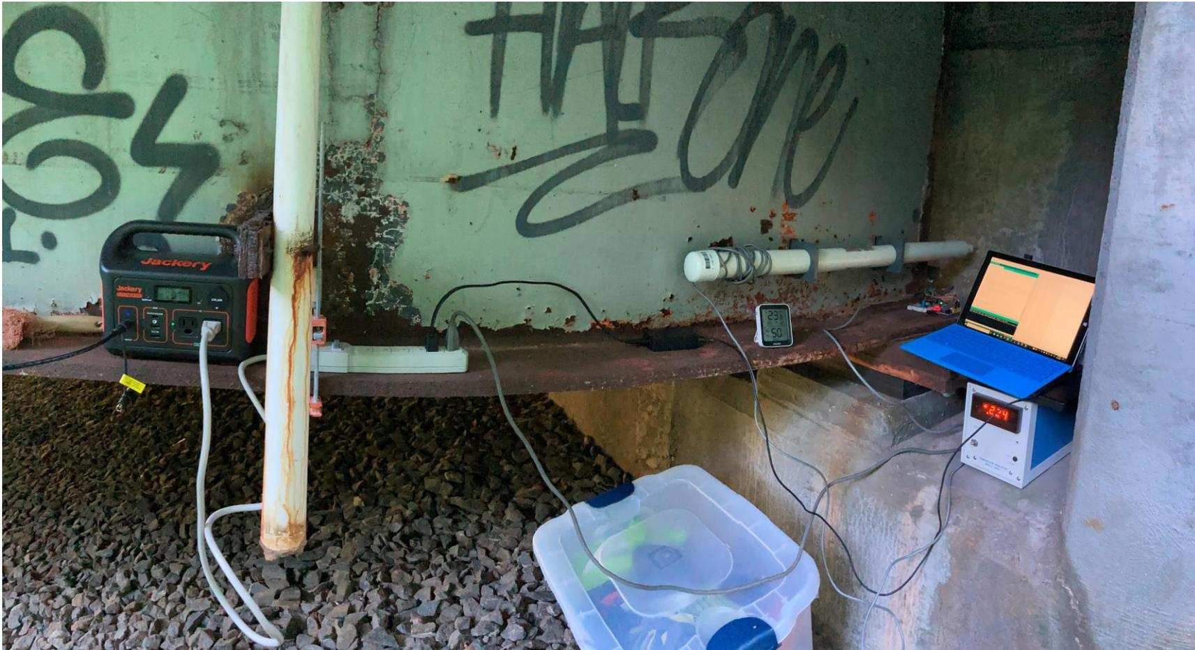
Figure 7. The second deployment on 6/14 using a Jackery power station with a solar panel – which supplied sufficient power to the system.
