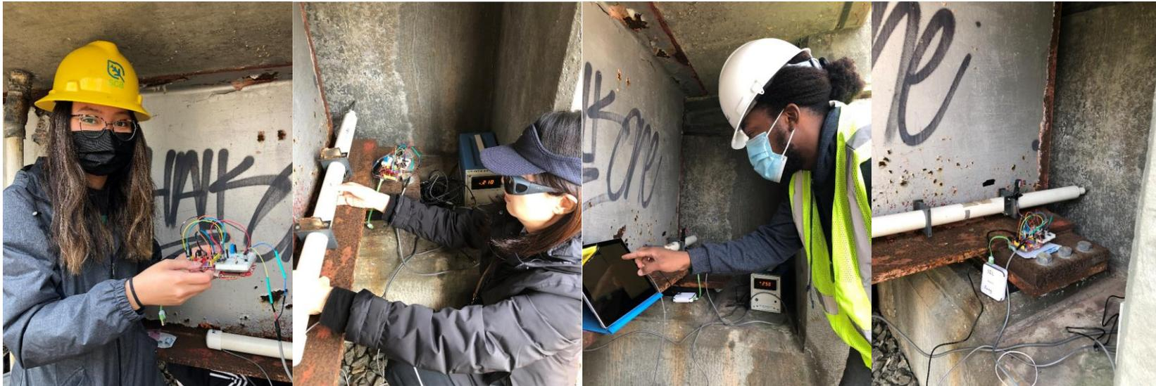
*Figure 3. Wireless Expansion Joint Monitoring Sensor Deployment on 4/25 (a) Daisy (undergraduate researcher) holding the Arduino, (b) Prof. Jang (PI) adjusting LVDT's level, (c) Pierre (graduate researcher) checking incoming data from the sensors, (d) installed sensing system.*
