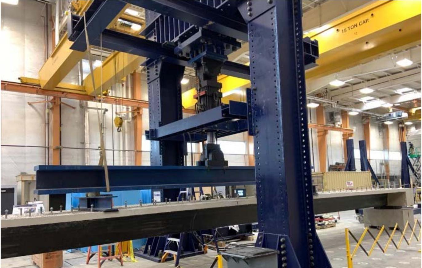
The double CT girder module under the loading frame
