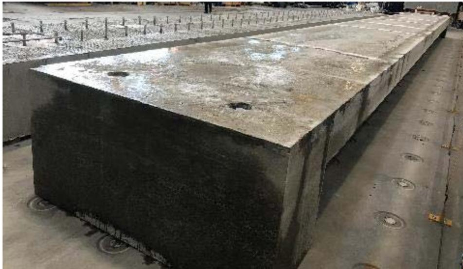
Creep Testing Girder Specimen
