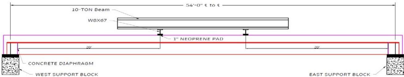
Test setup for Task 5
