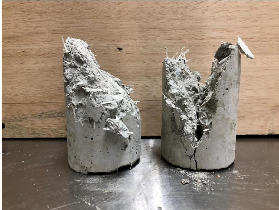
Figure 3 Concrete cylinder with fiber reinforcement following fracture testing
