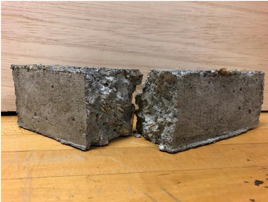
Figure 2 Concrete block sample following fracture testing
