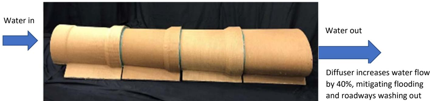
Figure 1: printed culvert diffuser (8.5 ft long, 2.5 ft wide) will be installed by Maine DOT to test protection against flooding.
