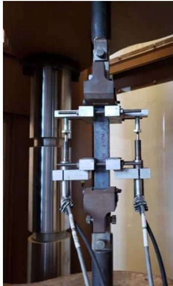
Fig:- Direct Tension Test Setup
