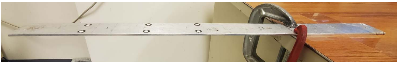
Figure 5. Cantilever beam setup.
