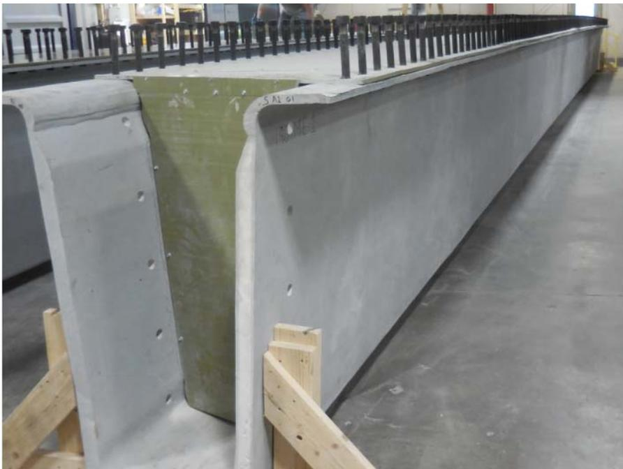
Fully infused, cured, and post-processed FRP tub-girder
