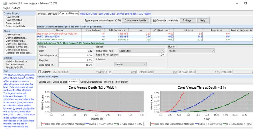
Figure 4: Analysis to compare time-dependent chloride concentration in (1) Normal concrete (No cementitious materials), (2) High volume fly-ash concrete (30% of fly ash replacement), and (3) Concrete with Silica Fume (10% of silica fume replacement)
