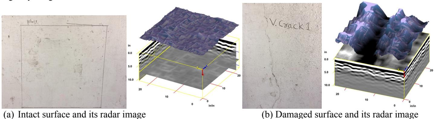
**Figure 1:** Photos and radar images of intact and damaged surfaces on a highway bridge in Lowell, MA.
