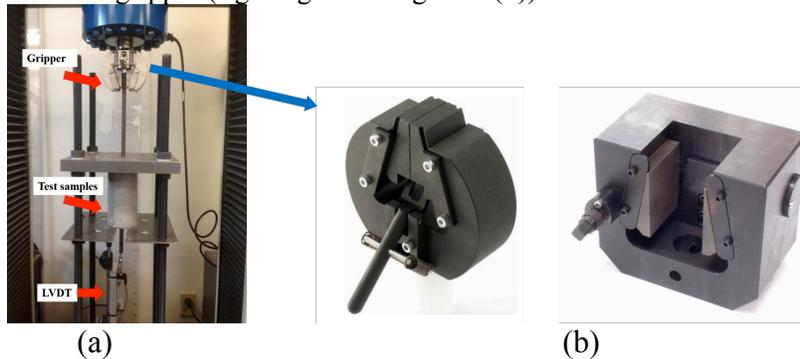
Figure 3: (a) Apparatus of pull-out test and (b) different types of grippers for the pull-out test.
