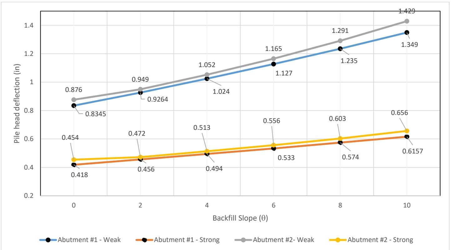
HP Piles head deflection vs range of slope (0-10%) for Bridge #38
