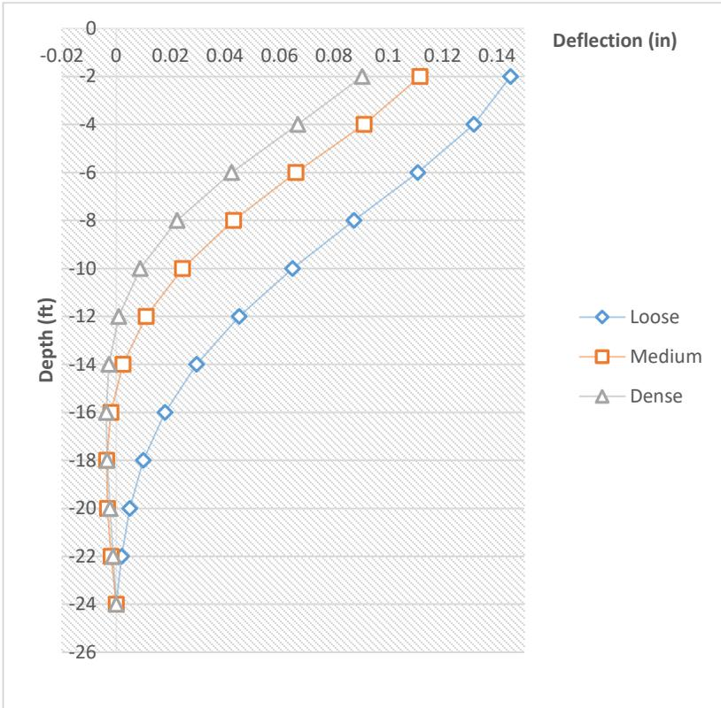
Deflection profiles for 25 ft. long HP piles for range of soil density
