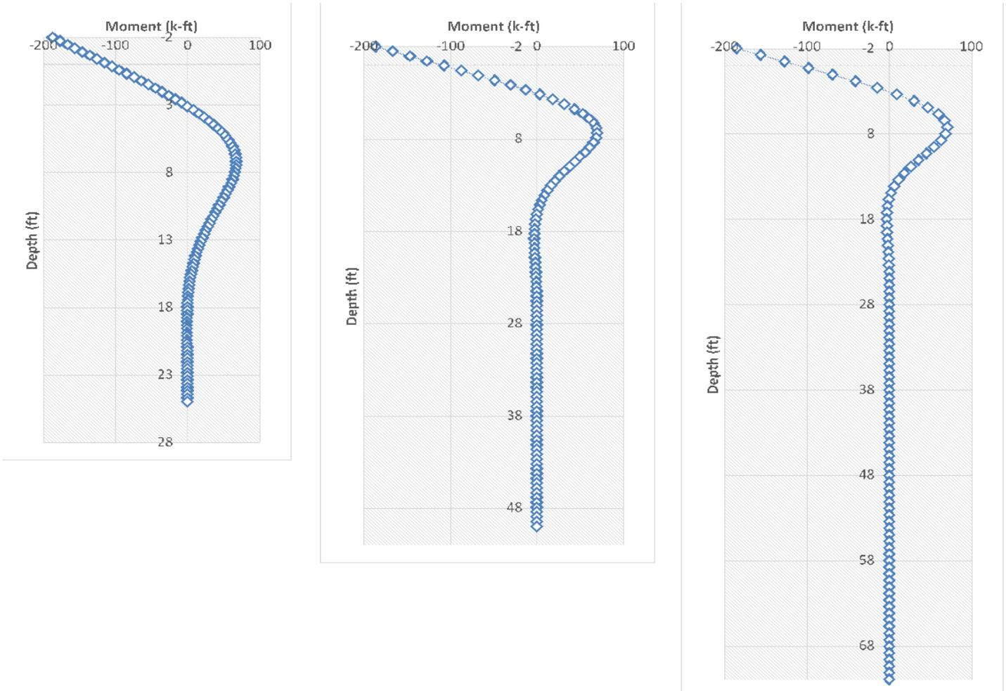
Moment diagrams for HP pile for range of pile length
