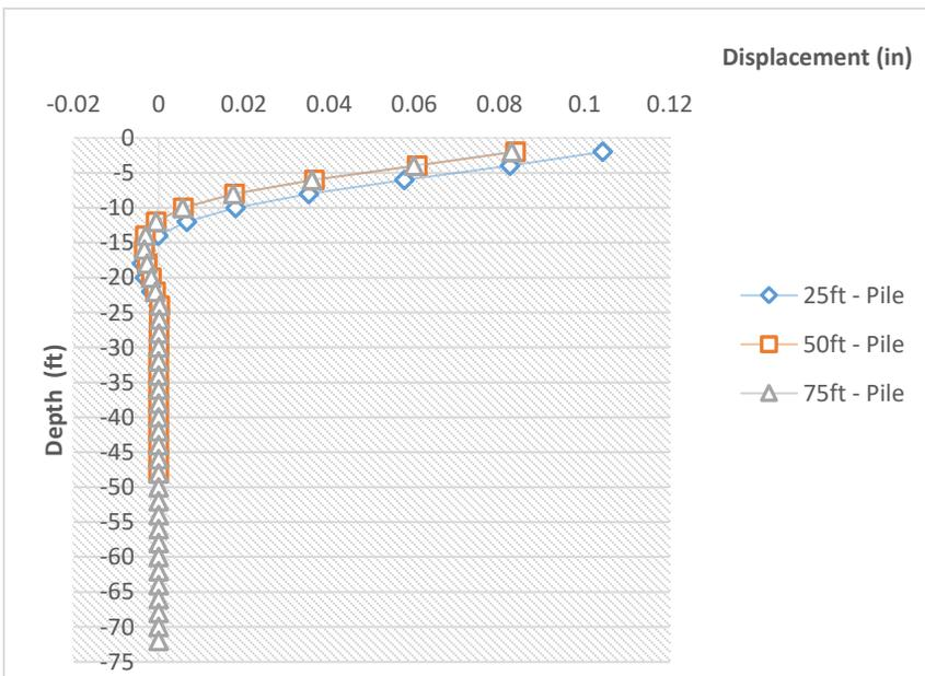
HP Pile deflection profile for range of pile lengths
