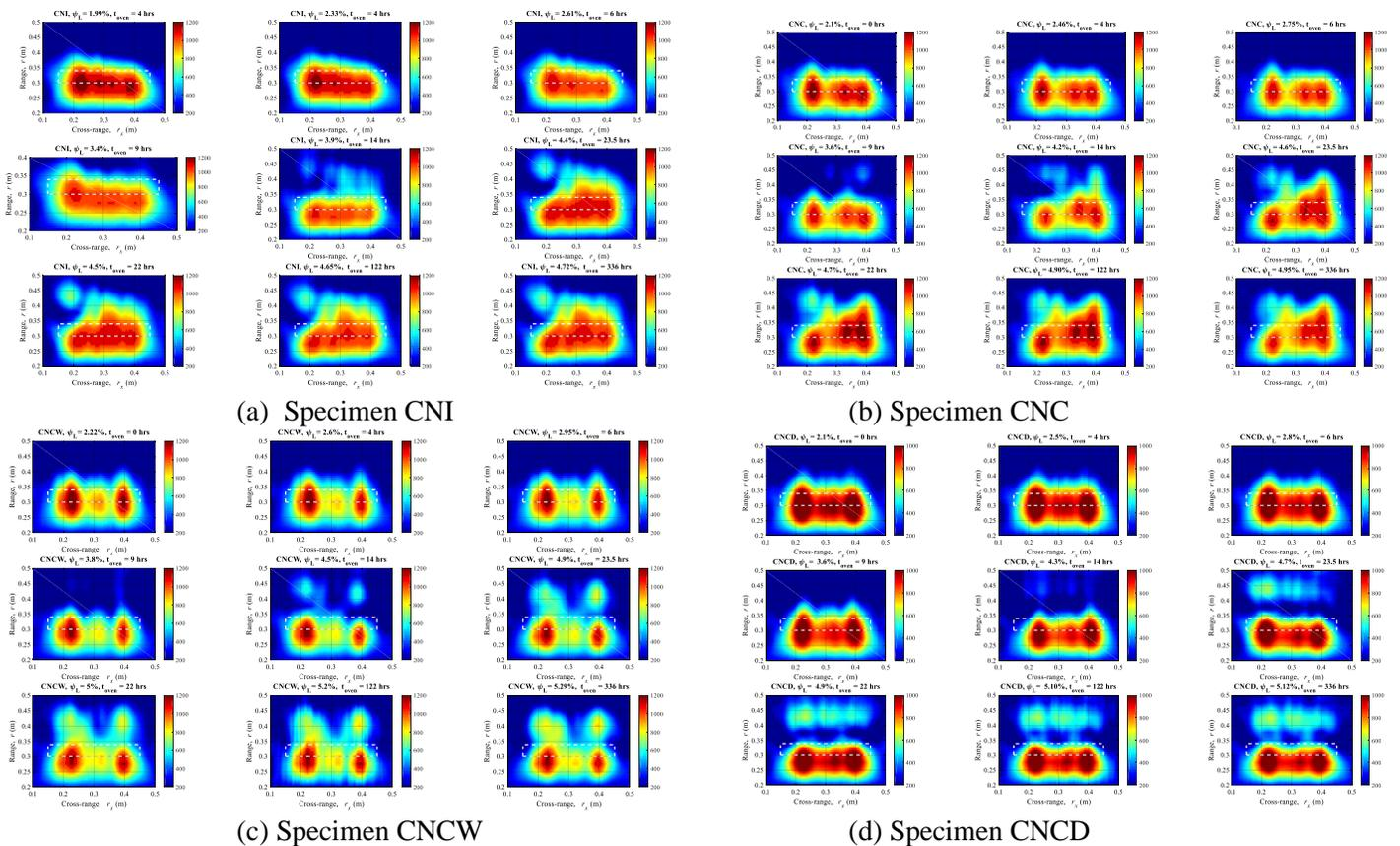
Figure 2. Oven-dried SAR images of all four concrete panels
