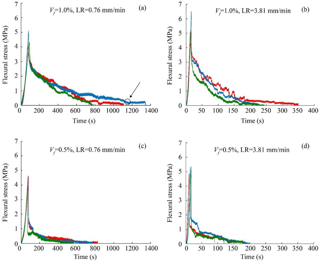
**Fig. 1.** Stress-time curves at 100 kHz of different steel-fiber beams during flexure (a) 1.0% fiber volume fraction, 0.76 mm/min loading rate; (b) 1.0% fiber volume fraction, 3.81 mm/min loading rate; (c) 0.5% fiber volume fraction, 0.76 mm/min loading rate; (d) 0.5% fiber volume fraction, 3.81 mm/min loading rate. Red, green and blue curves represented the three replicas in each group.
