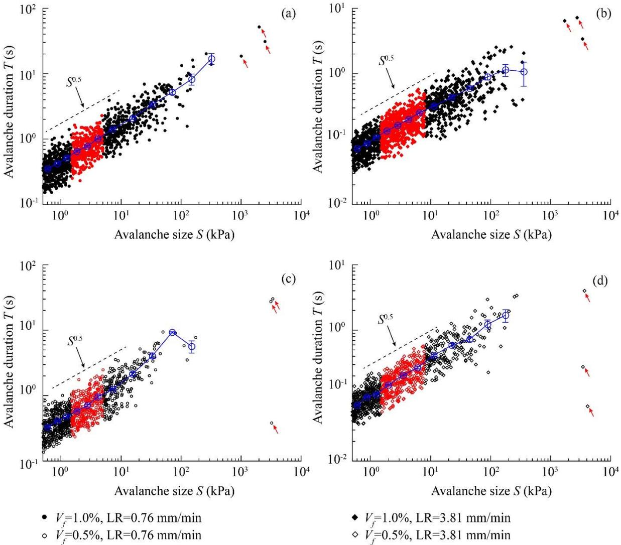
**Fig. 2.** Avalanche durations versus sizes for different groups (a) 1.0% fiber volume, 0.76 mm/min loading rate; (b) 1.0% fiber volume, 3.81 mm/min loading rate; (c) 0.5% fiber volume, 0.76 mm/min loading rate; (d) 0.5% fiber volume, 3.81 mm/min loading rate. Scaling regimes were highlighted in red.
