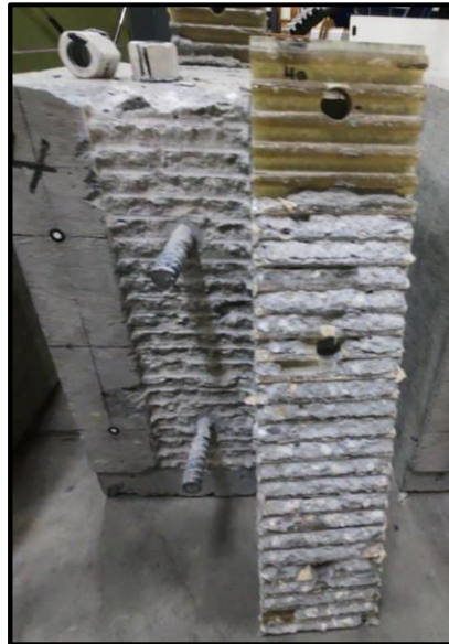
Figure 2-30: Shear Block 4 Inspection
