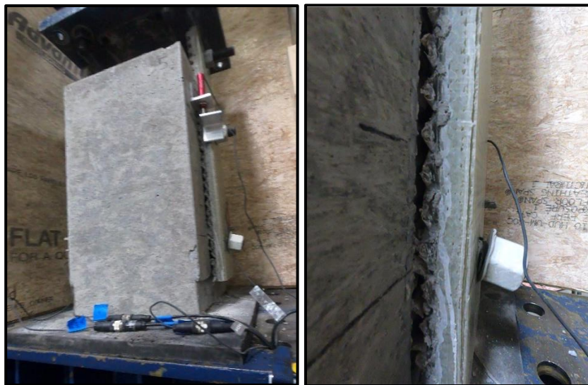
Figure 2-17: Failed Shear Block 5
