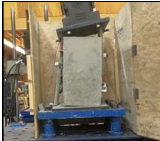
Figure 2-12: Shear Block 3 Premature Failure
