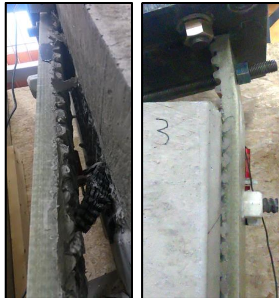
Figure 2-13: Failed Side (Left); Cracked Nut (Center); Bent Shear-Plate A (Right)
