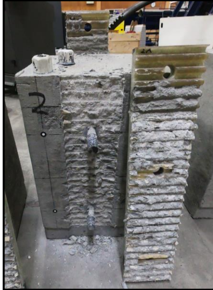
Figure 2-26: Shear Block 2 Failure
