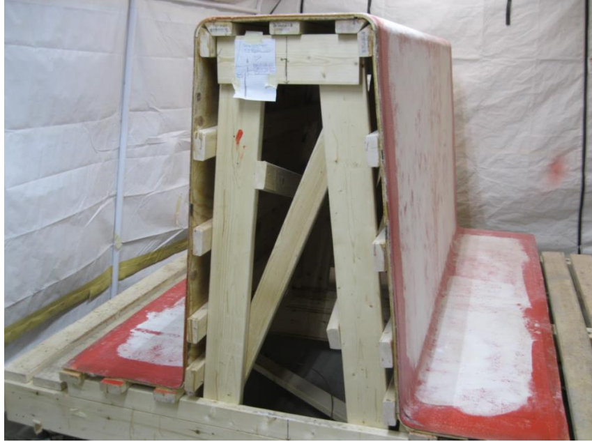
Figure 2: Male Mock-Up Girder Mold
