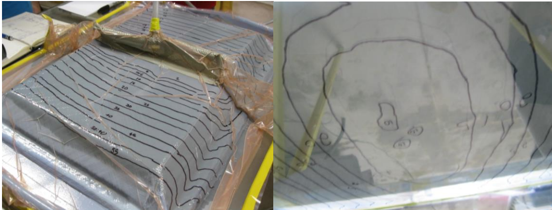
Figure 1: Test Panel Infusion to Calibrate Part Wet-out (Left: Panel Top; Right: Panel Bottom)
