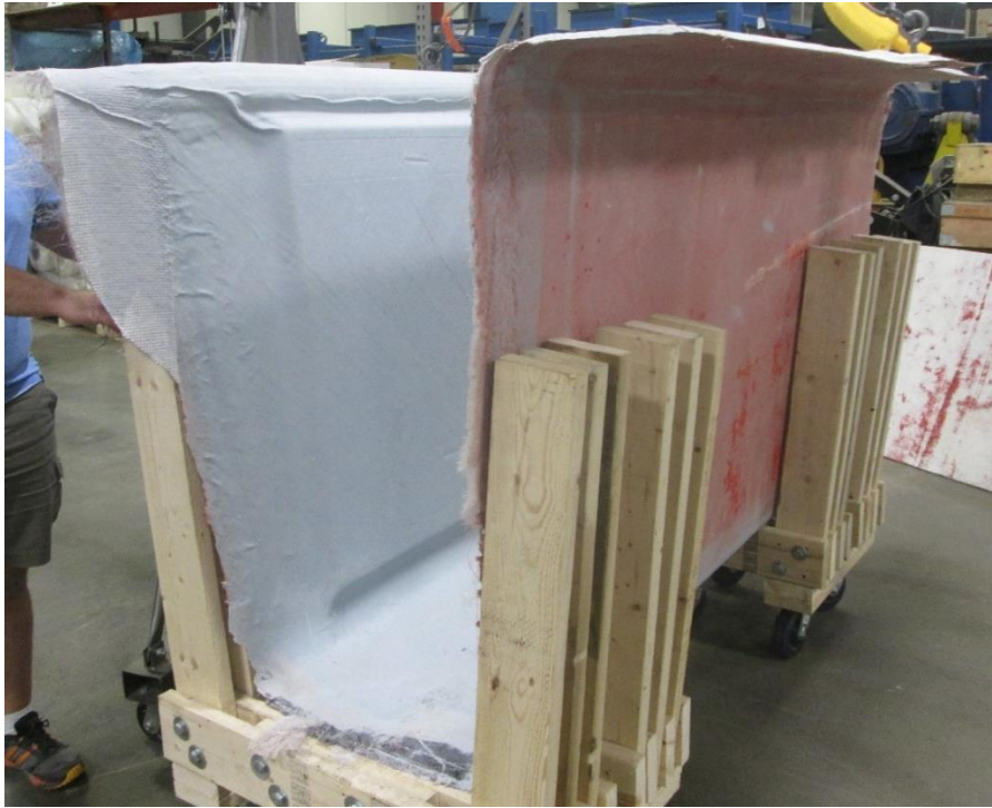
Figure 6: Infused, Cured Second Girder Mock-Up
