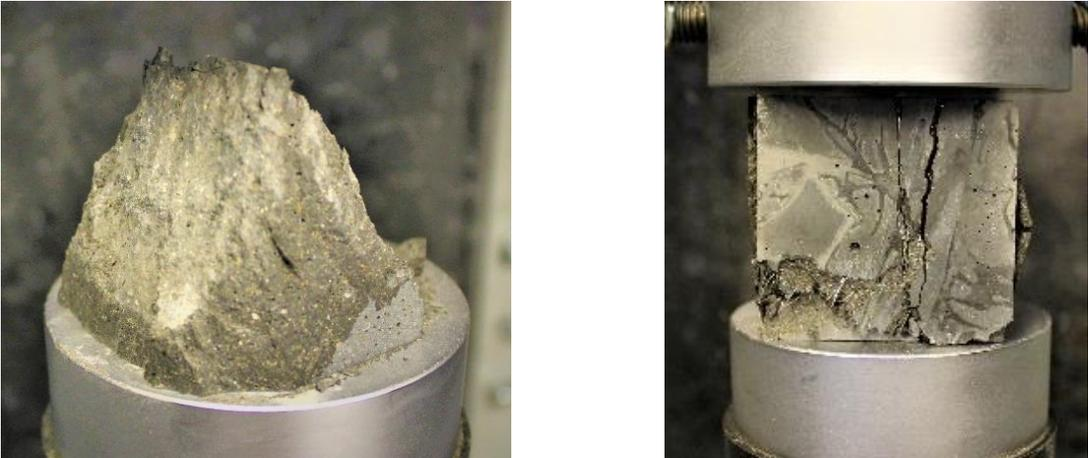
(a) Brittle failure (no steel fibers) (b) Ductile failure (with steel fibers)
