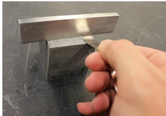
**Figure 9: a) Loading face preparation of cube on rotary grinder/polisher b) Planeness inspection**
