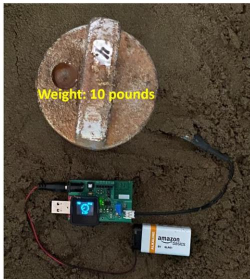
**Figure 20.** Pressure sensor buried in the sand box
