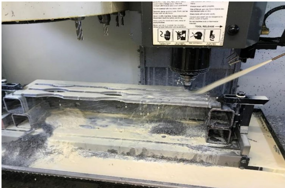
Figure 10: Fixturing of angle beams for coupon cutting
