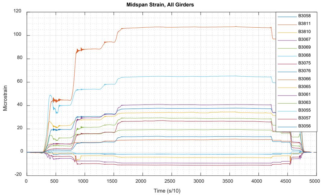
Figure 76: Bridge 2390 SBS\_U\_2\_1 Strains - Midspan
