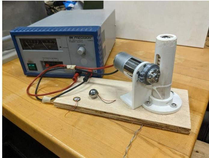
**Figure 1.** Rack and sector gear pinion steel ball tapper mechanism
