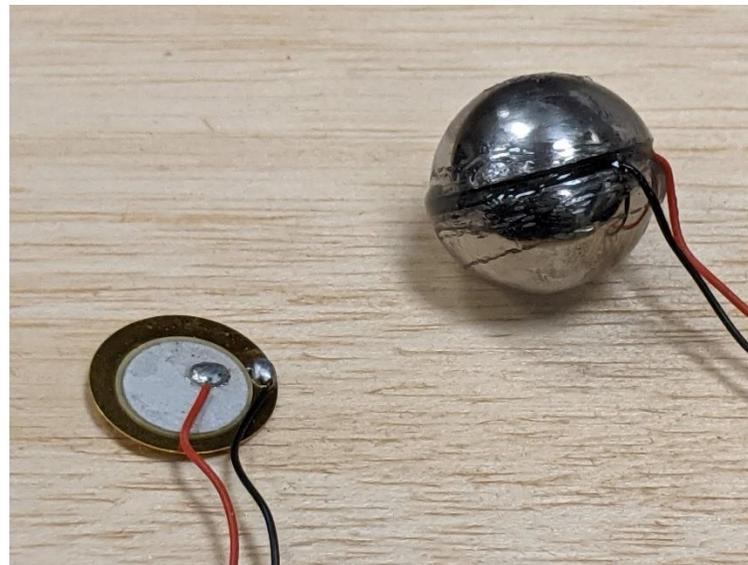
**Figure 2** Piezoelectric sensor ball and embedded sensor disk
