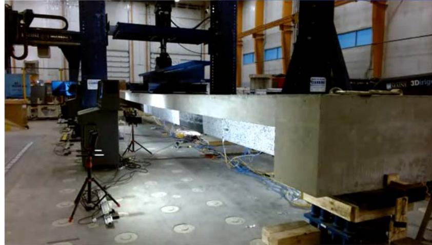
*Figure 1: CT girder under test frame*
