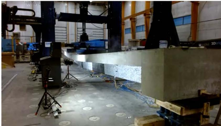
*Figure 2: CT girder post failure*
