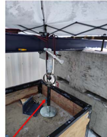
California Bearing Ratio (CBR) testing of carbonated soils
