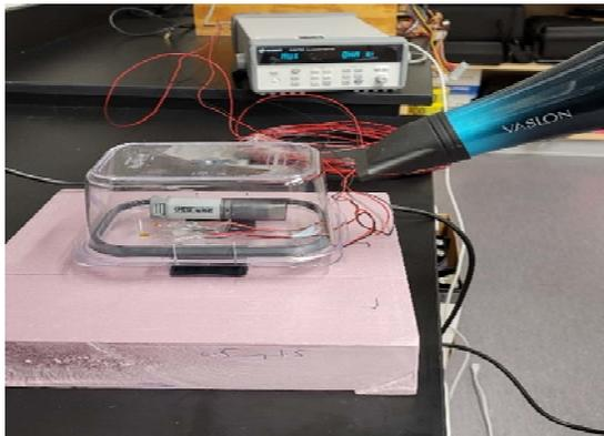
**Fig. 5.** Temperature test of strain gauges
