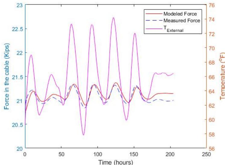
Figure 3 Comparison of predicted and measured force in left CFCC located in stay 10B
