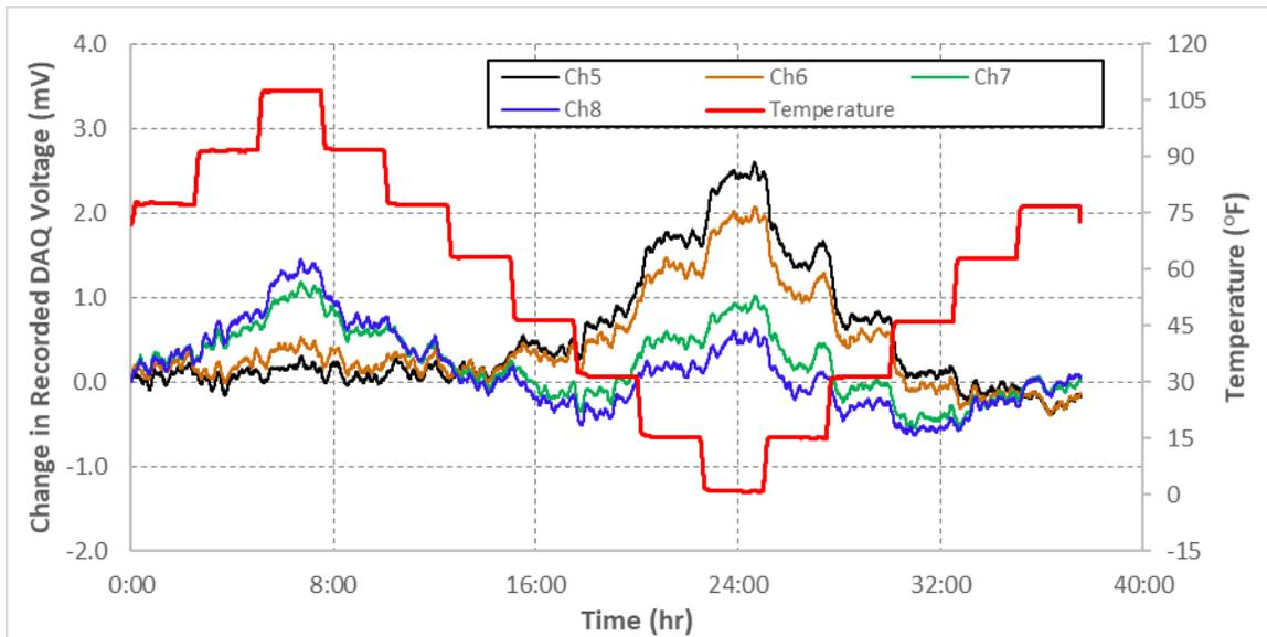
Figure 2: Temperature sensitivity results for the four voltage input channels of a V-Link 200 wireless DAQ module
