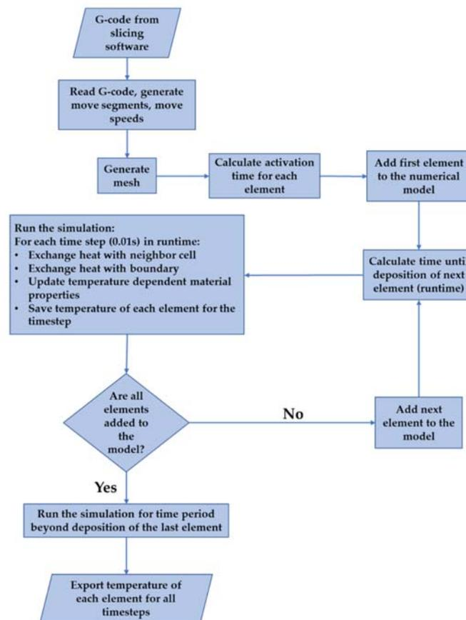
Figure 1. Flow chart of model developed to enable design of 3D printed parts
