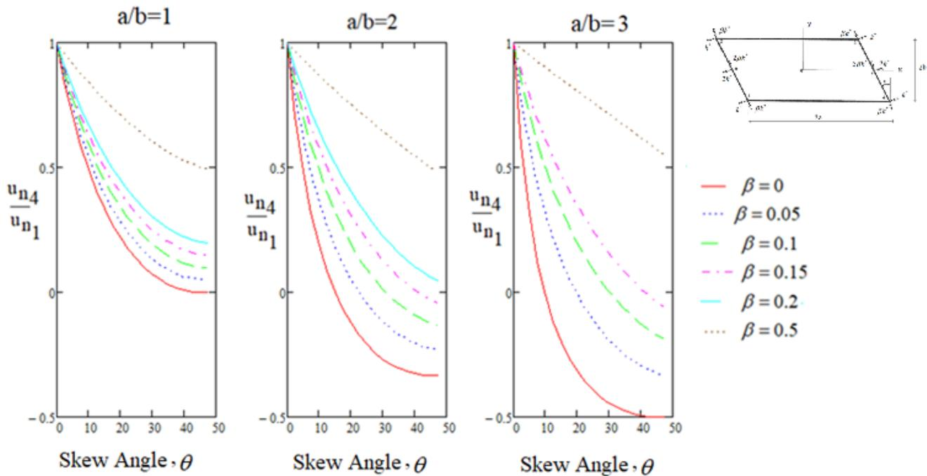
**Fig. 4** Variation of ratio of normal displacement at the acute corner to normal displacement at the obtuse corner of a skewed rigid plate with  $\theta$  for a representative range of  $a/b$  and  $\beta$
