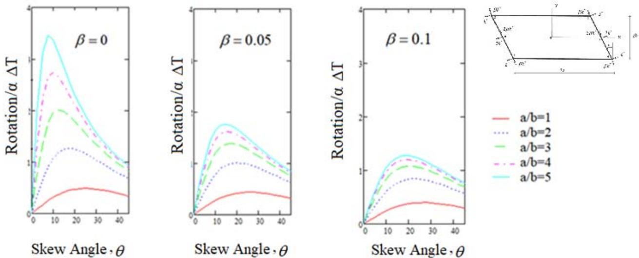
**Fig.2** Variation of in-plane rotation of a skewed rigid plate with  $\theta$  for a representative range of  $a/b$  and  $\beta$
