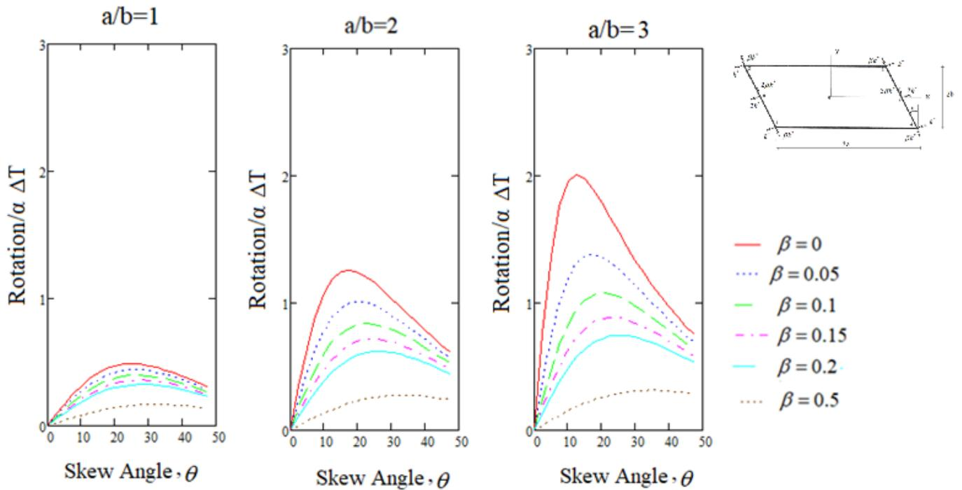
**Fig. 3** Variation of in-plane rotation of a skewed rigid plate with  $\theta$  for a representative range of  $a/b$  and  $\beta$
