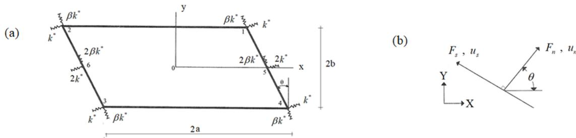
**Fig.1 (a)** Geometry of a skew plate and location of springs, **(b)** Orientation of normal and tangential axes
