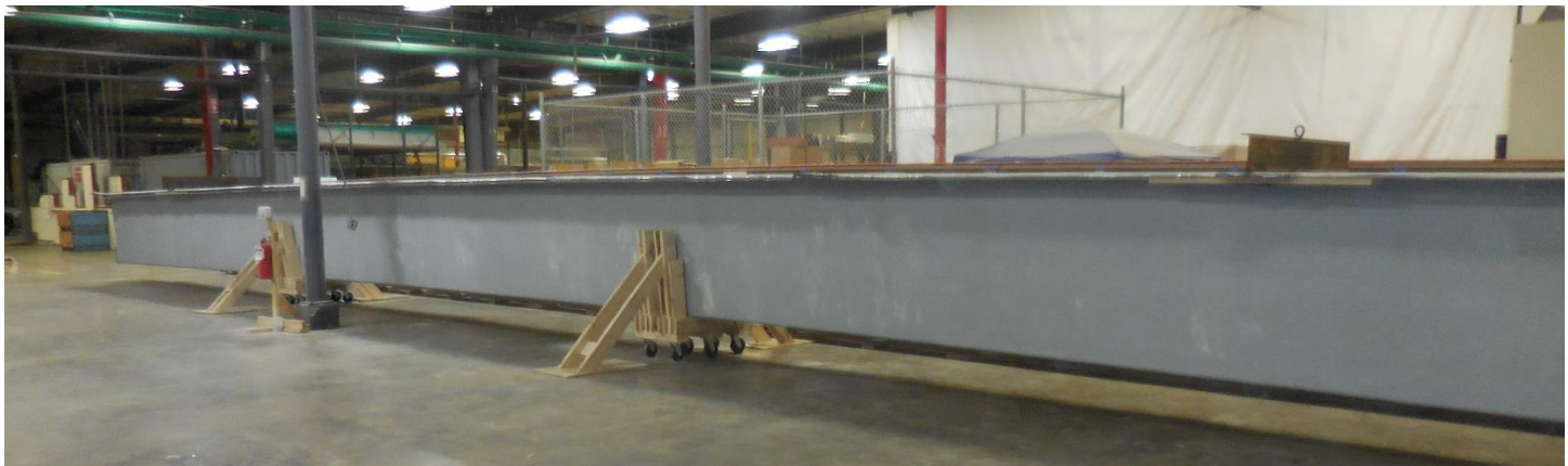
Fully infused and cured FRP tub-girder
