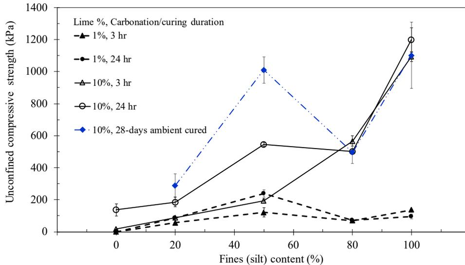
Figure 1. Effects of fine content on peak strength of carbonated and 28-days ambient cured (uncarbonated) lime mixed granular soil
