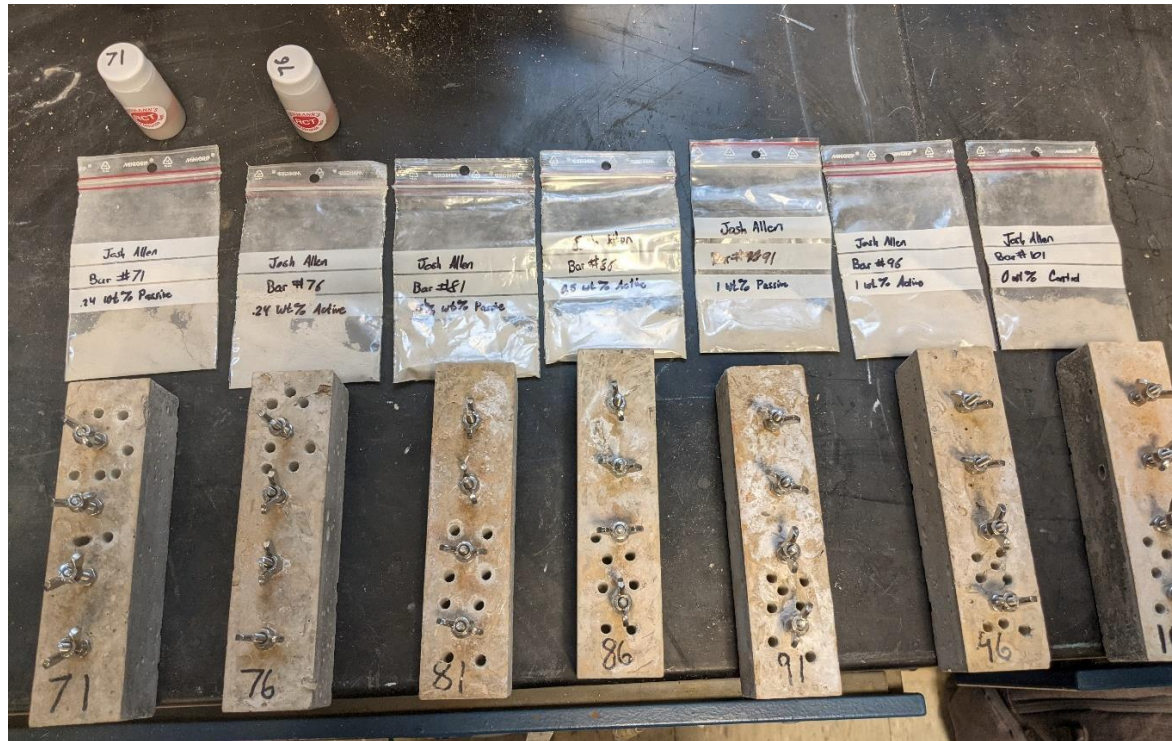
Figure 1. Rapid chloride testing of concrete beams with various levels of shrinking fiber content following long term salt water soaking
