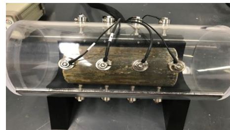
Fig:- Surface Resistivity Test Setup
