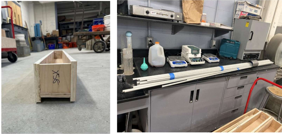
Figure 6. Wood Mold (left) and PETG Rebars Before Bending (right)
