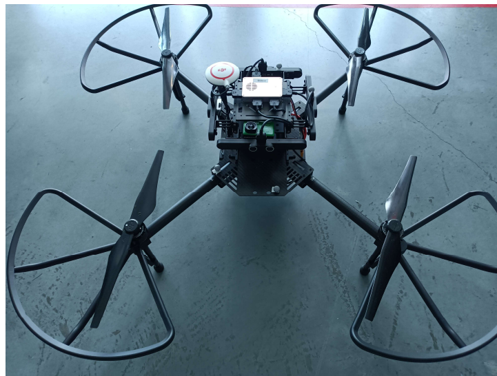
Figure 1: Drone setup with the guidance system and the camera.
